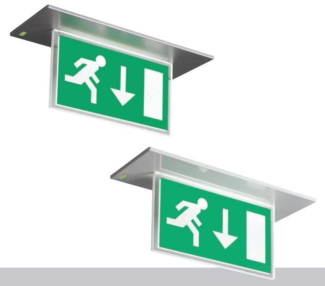
Briteblade is an unobtrusive recessed exit sign utilising a choice of traditional fluorescent light source or the latest LED technology. Installation is simple into either solid or suspended ceilings due to innovative rotating fixing arms that allow the fitting to pass easily into the mounting aperture on solid ceilings and a wishbone spring suspension system for ease of legend retention. A choice of white or silver trim finish makes Briteblade suitable for use in a wide range of applications.
