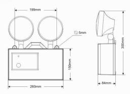
3 [+-] 2000 CO Order code EL40 2 x 21W 115 Lm Lead 12V - 7,2Ah Non maintained
